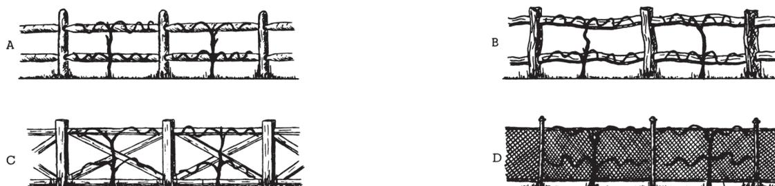
Figure 9. (A) Round poles for cross members. (B) Split rail cross members. (C) Cross members made of 2x4s. (D) Chain-link fence (twining of vines and tendrils in fence makes pruning difficult).
